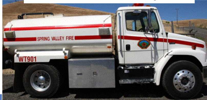
WT901 1994 Freightliner 2 axle Tactical water tender 2,000 gallons
